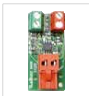
BUS INTERFACE BOARD For traditional photocell connection.
