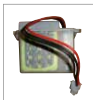
BATTERY KIT With recharging board.
