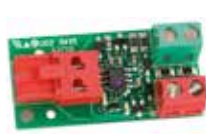
BUS XIB interface (for E045 or E024S control unit with non BUS photocell)
